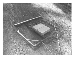
For driveways with the bump in the middle and 2 tire ruts this method below is just amazing. When you angle the unit as shown and remove one of the end plates, you can pull the material from the edge while riding on the center and quickly fill the ruts!
