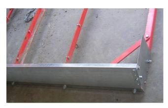
Loosen the side bolt furthest from the blade (Closest to the corner brace) on each side. Then loosen the 4 blade bolts to get enough clearance to slide the riser plates behind the washers. Tighten all the hardware once seated properly.
