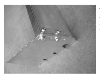
Assemble end plates to long plates with corner brackets and screws and nuts as shown. Leave loose for now. Be sure to place screws inside and **nuts outside**.
