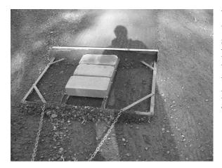
With the plates on, smaller material flows under and through the teeth while larger stones are waiting for a depression to call home. There is no flow over the top as the combination of angle on the plates and the build up of material will actually provide a small amount of lift when there are no depressions to drop material into.
