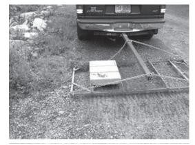
Shown from opposite side, this is a better way to go. The edge is being cut the most and moving the material toward the middle. Note that the cutting stops just past center. Adjust weighting and angle for the conditions is the rule. This is also best for weed removal. With a little practice, you will get better results.
