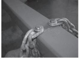
Simply take up enough links each side of the chains so it has some slack and insert washers and clevis pins in the holes. **Note:** Orient the links as shown so that the loops are on the same side of the link you use
