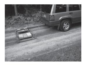
This is what you don't want to do. More material is being removed from the center to fill the rut than the edge. If you weight to one side, or partially to one side and angle slightly like above you will use mostly edge material to fill the rut. If you have a very flat driveway, this is not so important. But if you have a sloped one, you will create a washout next rain if you make the middle lower than the edges!!
