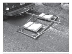
This is OK for really packed surfaces but notice that the center is cutting more than the edge.
