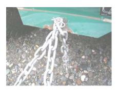
To change the length on one side to angle the unit, put to links on one side of the connecting link as showns. Altering chain length to angle unit will be discussed in the use and operation section.
