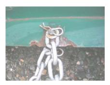
Place the unit about 18" from the rear of the vehicle at the desired start point. Remove one hairpin and washer and put up through the hole on the vehicle. Then put chain, washer and hairpin to connect.
